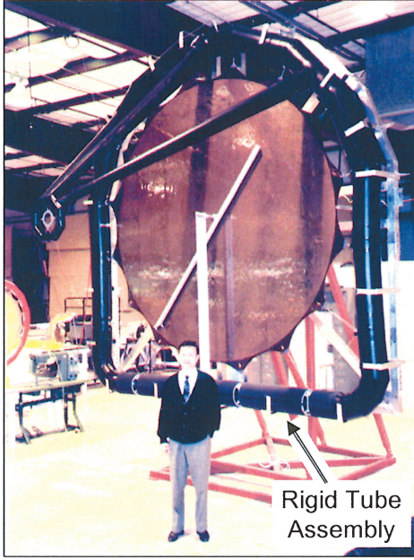
Fig. 2 Three-meter Ka-band inflatable reflectarray antenna.
